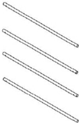
4 x pipe Ø25,4 x 1,0 mm L = 1000 mm
